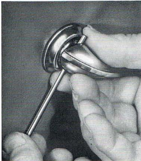
Fig. 67. Removing internal door handle.
