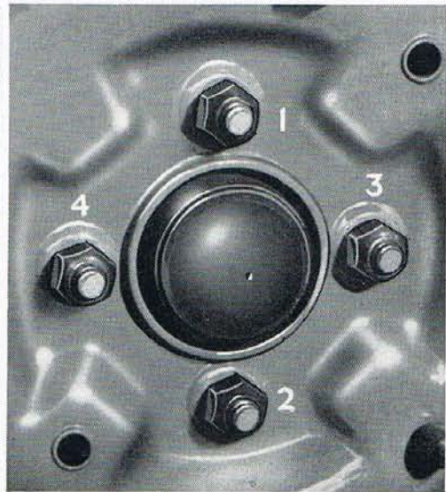
Fig. 35. Roadwheel nut tightening sequence.
