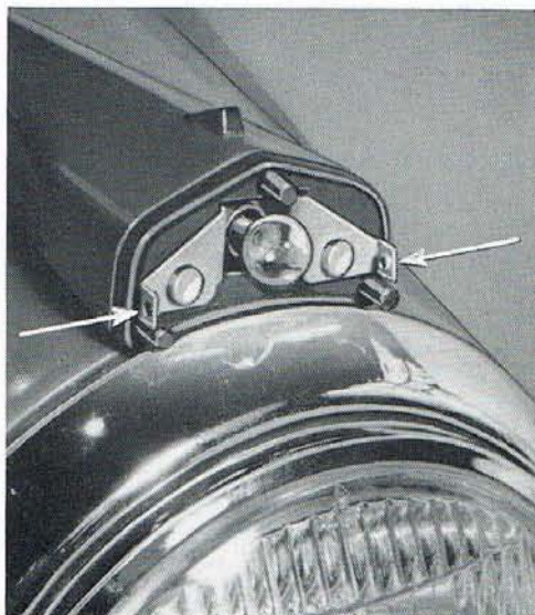
Fig. 52. The side lamp with glass and rim removed.
