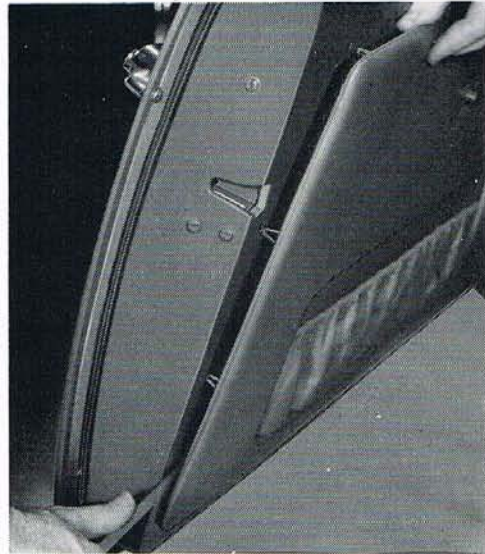
Fig. 68. Removing the door trim panel.
