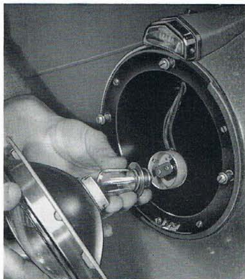
Fig. 51. Replacing the headlamp bulb.
